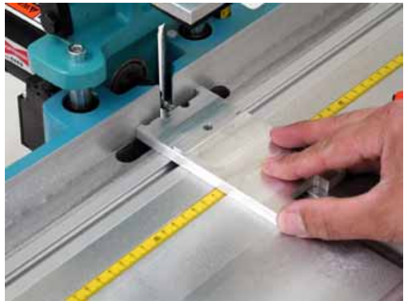
Square-stop used as set-up jig (center notch = W2)
